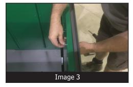
**3.** Slide a corner bracket between the BearGuard and the front corner of the Razorback (See Image 4). One at a time, insert the four 1/4" x 1" carriage bolts through the Bear Guard, the corner bracket and the Razorback (See Image 5) and put washer and NyLock on each bolt. DO NOT TIGHTEN THE NUTS!
