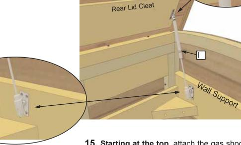
**Important**: Gas Shocks will be fully extended when initially installing.
