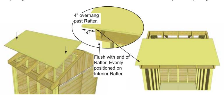
**43.** Starting in front corner, !ocate 5/8" x 78" x 32 1/4" Plywood Roof Section and place on top of Roof Rafters. Position so Plywood overhangs outside Rafter by 4". At bottom of Rafter, Roof Panel should be flush with Rafter end.
