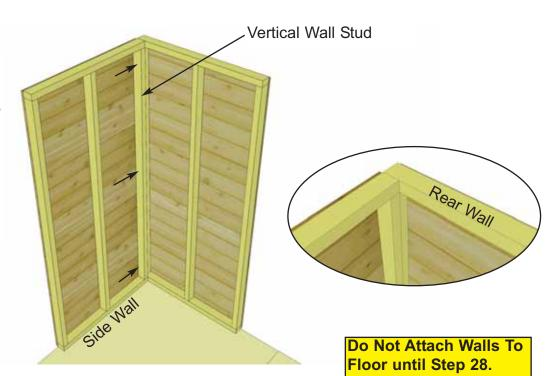
**17.** With the corner wall attachment complete, position a second side wall panel in place.
