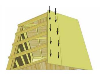
**44.** When Plywood is correctly positioned, fasten down into Roof Rafters with 10 - 1 1/4" screws. Locate 78" x 13" Plywood Roof Piece and position as illustrated above. Attach to Roof Rafters with 10 - 1 1/4" screws.
