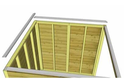
**26.** Complete remaining Side and Rear Top Plate attachments as per **Steps 24-25**.
