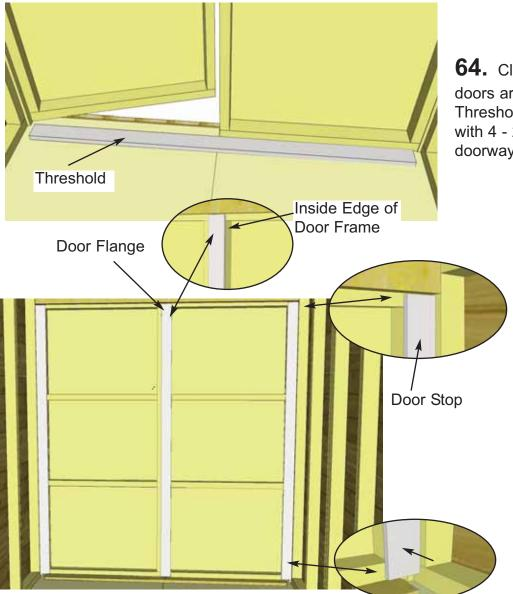
**64.** Close both doors and align so doors are straight. Attach Door Threshold (2 1/2" wide x 62 1/2" long) with 4 - 2" screws centering between doorway.
