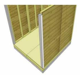
**22.** Attach Door Jamb to vertical wall stud with 4 - 2 1/2" screws. Complete both Door Jambs.
