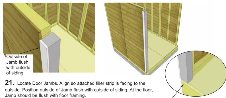
Jamb should be flush with floor framing
