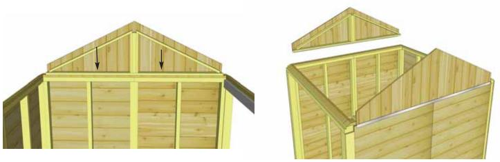
**29.** Temporarily attach Gable to walls and top plate with 2 - 2" screws. Screw from the bottom of gable framing down into Top Plate and Wall. Gables may need slight adjustment in **Step 40** and then be completely attached with an additional 6 - 2" screws. Position 2nd Gable on side walls.
