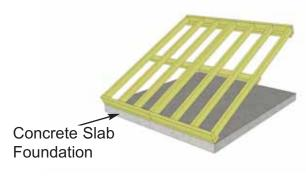
**9.** With Floor Runners attached, carefully flip the floor over and place on your foundation. **Caution-** you will need 2 people to assist you. Be careful when laying floor down not to bend or twist floor. When in place, level floor completely.
