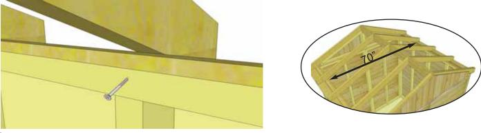
**41.** Secure Rafters to Top Wall Framing with one 3" screw per rafter. Screw through Wall Frame at an angle. Have two helpers push the Front and Rear Walls at the top from the outside of shed until inside to inside measurement between the Top Plates is 70".
