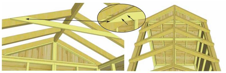
**42.** The **Roof Gusset** is positioned on center rafter. When correct, slide gusset up, use level to square gusset and attach to rafter with 4 - 1 1/4" screws. **Pilot hole Gusset to prevent splitting.**
