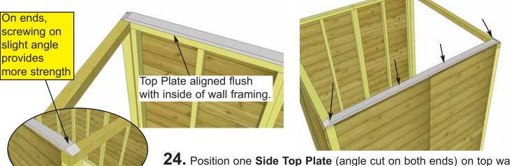
**24.** Position one **Side Top Plate** (angle cut on both ends) on top wall framing. Top Plate should be evenly spaced from front to back and aligned flush with the inside of wall framing. Attach into wall framing with 4 - 2" screws.
