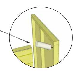
**16.** Position side wall into place on plywood floor. Butt both vertical wall studs of side and rear walls together and attach with 3 - 2 1/2" screws. Screw at the bottom, middle and top of stud to secure properly.
