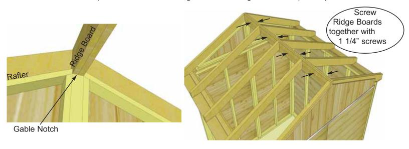
**39.** With Ridge Board locked into gable notch, align Ridge Boards so they are flush together and secure them with 8 - 1 1/4" screws. **Important**- if there is a gap between Ridge Boards, try pushing rear wall and Door Header closer together from outside. Walls should be 70" apart at top from inside of wall plate to wall plate.
