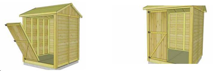
**59.** Next, position and secure the Double Doors. Starting with **Left Side Door**, position so there is a 1/2" gap on bottom and approximately 3/8" on the side. Use a spare Shingle to shim door in place at the bottom.
