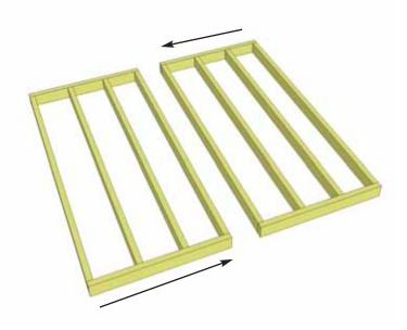
**3.** Lay out both completed **Floor Joist Frames** as illustrated at left.
