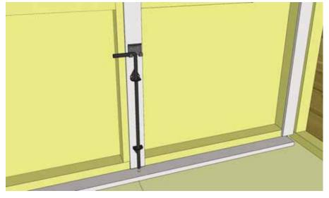
**66.** The **Interior Cane Bolt** will be attached to Vertical Door Flange. To position Cane Bolt correctly, attach to flange first, close doors and mark hole to house Cane Bolt Rod. Open doors and drill hole where previously marked with 1/2" bit. Use hardware provided in each kit to complete installation of all hardware.
