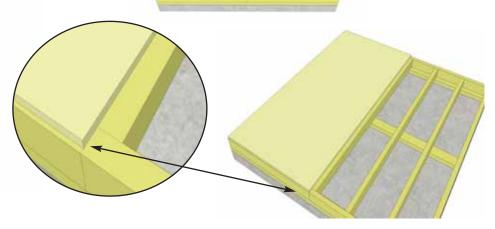
**10.** Position **Plywood Floor** pieces (2) on top of completed floor frames. The Plywood is cut slightly smaller than floor framing. Keep plywood seams tight.
