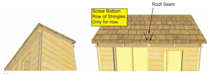
**39.** With Roof Panel aligned, screw panels down to center rafter with 2 - 2 1/2" screws in the bottom row of shingles. (1 screw per panel).
