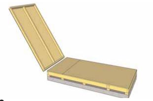
**10.** Starting on Side, position a **Solid Wall Panel** on top of plywood floor. The Wall Panel bottom framing will sit flush with floor framing. Wall siding will overhang the floor. **Important:** Make sure all walls are aligned in their upright position. If not ,water may leak into your shed. Unsure if panel is facing up or down? Recently attached Bottom Plate is on bottom of panel.
