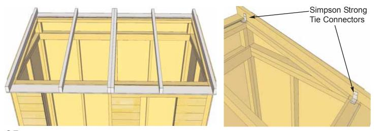
**35.** With Rafter Section correctly aligned, secure rafters to walls using **Simpson Strong Tie Connectors**. Start with outside rafters and secure 2 Strong Ties with 1 1/4" screws. Screw into Wall Extension Framing at the rear and the Wall Panel top framing at the front. Complete both sides.
