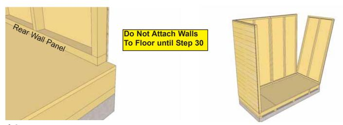
**14.** With Rear Wall Panel in place, position other side wall panel on floor as per **Step 10 & 11**.
