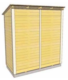
**56.** Attach **Middle Trim** - 1/2" x 2 1/2" x 88 3/4" where wall panels come together at rear seam. Attach with 8 - 1 1/4" finishing nails aligning flush with bottom skirting.
