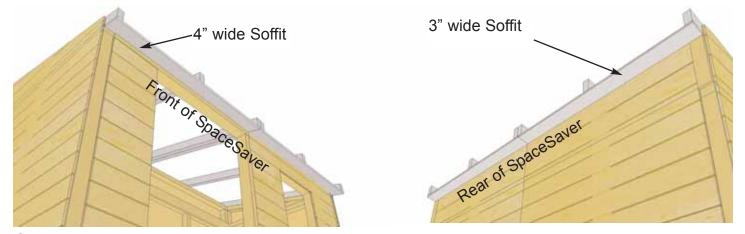
**34.** When Rafter Section is positioned correctly, both Front and Rear Soffits will sit approximately 1/8" away from wall siding. This can vary slightly.
