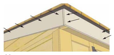
**63.** With Side Angle Cut Facia correctly aligned, attach Front Facia to rafter ends with 6 - 1 1/4" finishing nails per piece. Attach Side Angle Cut Facia to plywood ends with 4 - 1 1/4" nails. Attach next piece of Front Facia.
