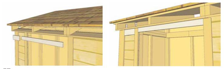
**57.** To complete trimming of your SpaceSaver, attach both the **Horizontal Door Trim** and **Horizontal Narrow Wall Trim** with 4 and 2 - 1 1/4" finishing nails. Place trim flush up against Soffit.
