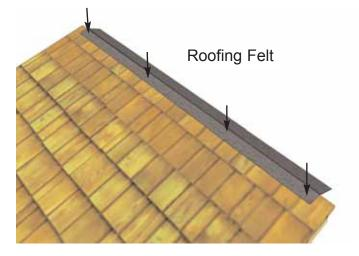
**65.** Locate 8" wide x 96" long **Roofing Felt** and make a 3 3/4" wide fold along the 96" length. Place on top of roof shingles evenly spaced between outside rafters and secure with 4 - 1 1/4" nails.
