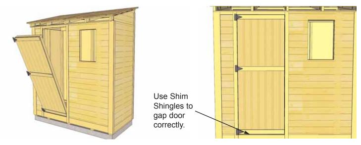
**59.** With Hinges attached, position door in opening. Use Shim Shingles to establish gap.
