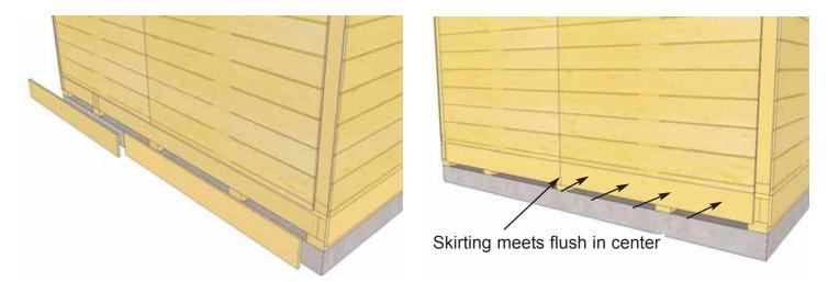
**45.** Rear skirting pieces will meet together in the center. Secure with 4 - 1 1/4" finishing nails per piece.
