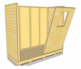
**15.** Secure side wall panel to rear wall panel as per **Step 12**. Next, locate **Window Wall Panel** and place in front corner.
