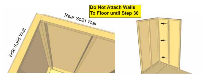
**12.** Butt both vertical wall studs of side and rear walls together and attach with 3 - 2.5" screws. Screw at the bottom, middle and top of stud to secure properly. **Note: Drill pilot holes in studs to prevent splitting**.
