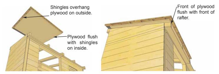
**37.** Correctly orientate Left Side Roof Panel with shingles overhanging the plywood on the outside left and shingles flush with plywood on the right. Place on rafters with front of plywood flush with front of rafter. **Note:** trimmed shingles on roof panel to back of shed.
