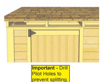
**61.** Make sure Door Panel is aligned evenly at top and edge. When aligned correctly, attach top and middle hinges to narrow trim with hinge hardware provided.
