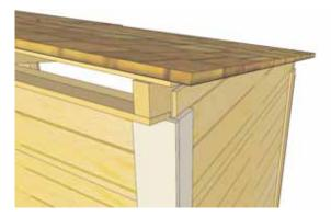
**55.** To completely trim out rear corners, locate **Rear Trim** -  $1/2^{\circ} \times 2 1/2^{\circ} \times 88 3/4^{\circ}$  and a **Rear Corner Trim** -  $1/2^{\circ} \times 4 1/2^{\circ} \times 88 3/4^{\circ}$ . Align and attach as per **Step 54**.
