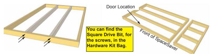
**2.** When correctly positioned, attach each Joist with 4 - 2 1/2" screws (2 per end). **You can find the Square Drive Bit for the screws in with the Hardware Kit Bag.**
