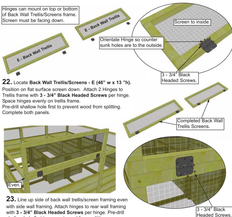
with 3 - 3/4" Black Headed Screws per hinge. Pre-drill shallow hole first to prevent wood from splitting.
