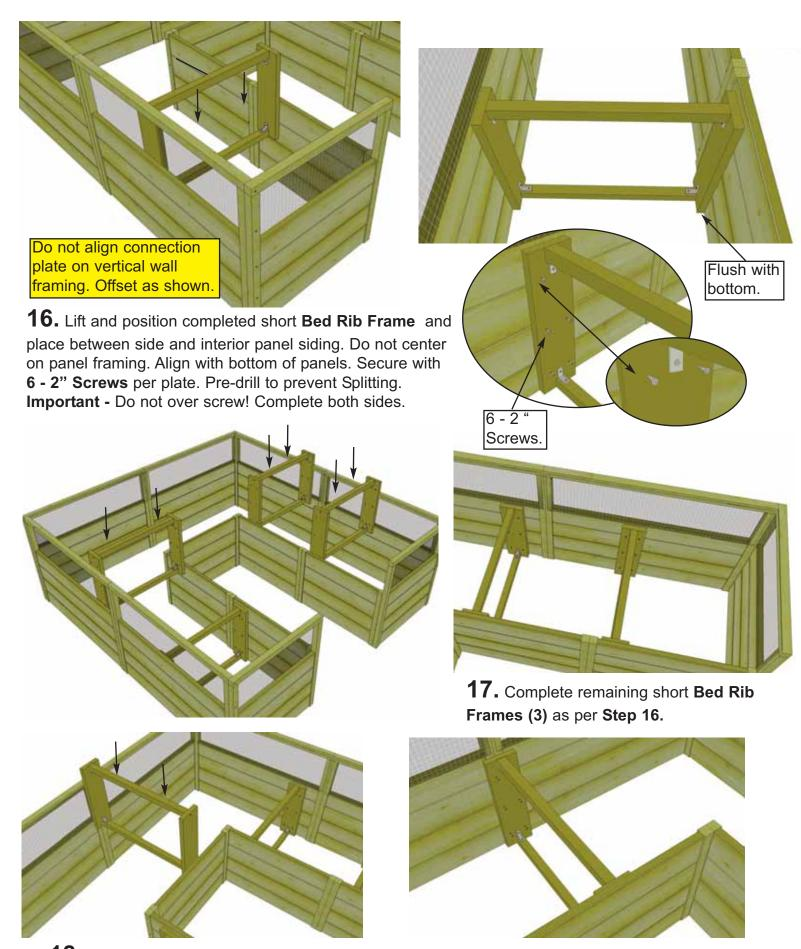
**18.** Lift and center completed longer **Bed Rib Frame** on rear and end interior panels. Align with bottom of panels. Secure with **6 - 2" Screws** per plate. **Important -** Do not over screw!
