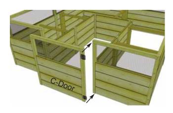
**19.** Locate **Door Panel (Part C) - 30 5/8" w x 31 1/2" h)** and position on flat surface screen down. Attach both hinges to door panel with **3 - 3/4" Black Headed Screws** per hinge. Space hinges evenly on door frame. Pre-drill shallow hole first to prevent wood from splitting.
