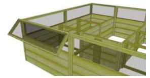
**24.** Complete attachments of both back wall trellis/screens to rear wall framing. Confirm screens can move up and down smoothly. Adjust if necessary.
