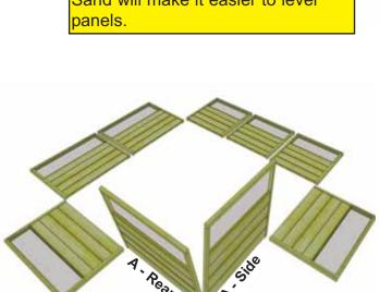
2. Starting in rear corner, position Rear and Side Panels (Part A) - 46" wide together so framing is flush at top and sides. When aligned, attach frames together at top with 1 - 2 1/2" Screw. Use Wood Clamp to hold frames together. Pre-drill rear frame first with 1/8" diameter bit to prevent wood from splitting.
