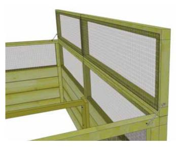
25. Lift trellis/screen into the up position. Screw male portion of Eye Hook into trellis/screen side framing and female piece into side framing of side wall. Do a dry run first to confirm correct position. Complete both sides.
