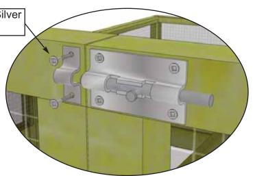
**26.** Attach **Barrel Bolt** (male and female pieces) to side framing of trellis/screen. Use 6 - 3/4" Silver screws. Pre-drill shallow hole first to prevent wood from splitting. Do a dry run first to confirm correct position. Barrel Bolt may be silver/black.
