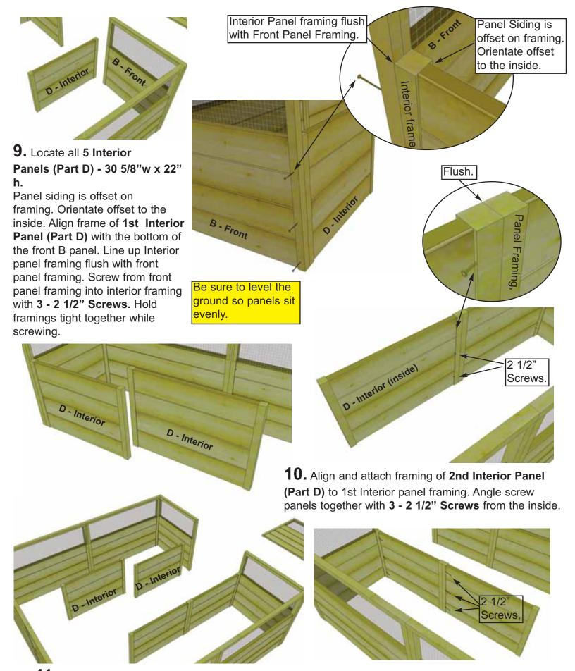
11. Align and attach framing of 3rd and 4th Interior Panels (Part D) as per Steps 9 & 10. Angle screw panels together with 3 - 2 1/2" Screws from the inside.
