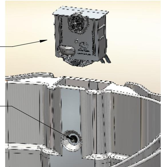
Push in on this button and lift out latch assm.
