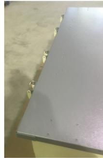
8. Install the hinge bolts. To do this it is important to install one hinge bolt at a time. There are a couple
