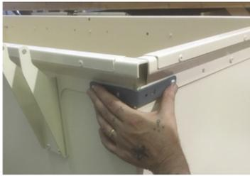
5. Install the four corner brackets on each of the top corners of the bin. Using four 1/4” x 3/4” carriage bolts per corner bracket, insert the bolts one at
