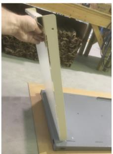
the corresponding slots on one side of the base. Ensuring that the tabs are fully engaged (if not fully in place, the tabs or side panel could distort), gently lift the side panel until vertical. There is a built in catch that should hold the panel in place. After the first side is in place, install the other side the same way.
