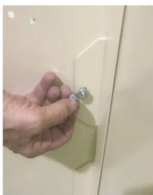
4. Install the Front Panel in the same way as the Rear Panel. Insert the remaining two 1/4” x 5/8” carriage bolts, and put on the washers and nuts.
