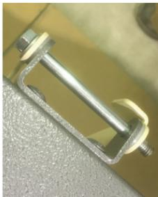
of steps for each hinge bolt: a) place a 5/16” nylon washer on each side of the lid hinge brackets, between each flange of the Rear Panel hinge bracket. b) place a 5/16” washer on the 5/16” x 3 1/2” bolt, and slide the bolt through hinge bracket holes, ensuring the nylon washers stay
