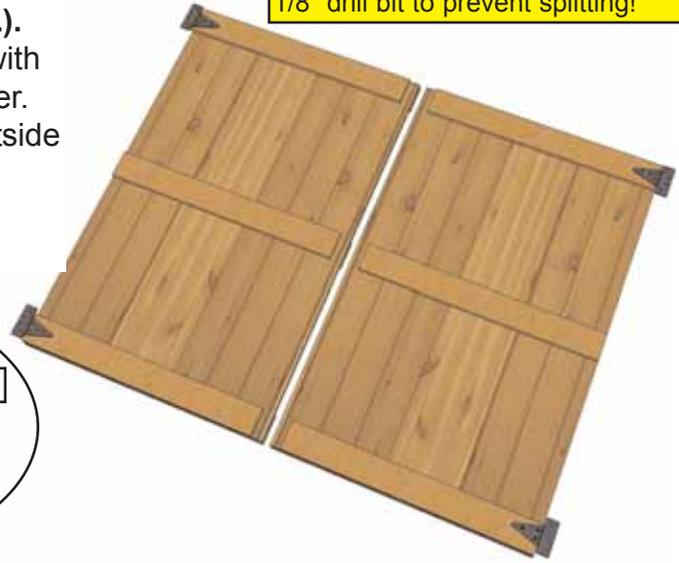
**20.** Line up pre-drilled holes in hinge and door and slide bolt through. Tighten bolt using 3/8" socket or wrench. Finish hinge by securing with **2 - 3/4" Black Screws (G)**. Drill shallow depth pilot holes first to prevent wood from splitting. Complete both doors (4 hinges).
