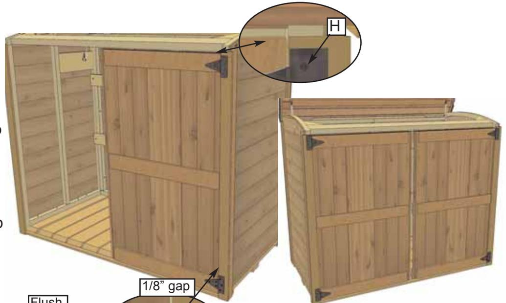
**Drill 1/8" pilot holes for 2" screws to prevent wood from splitting.**
