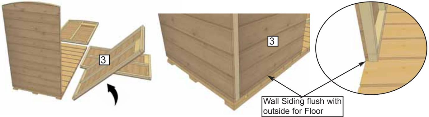
**4. Lift up a Rear Wall (3)** and orientate the wall as shown above. At the bottom, align wall siding even with outside of the floor. At the top, align wall siding flush with framing of side wall. When correctly aligned, attach wall frames together with **3 - 2 1/2" screws (A)**. Screw on a slight angle to penetrate the side wall framing best.
