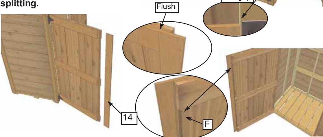
**22.** Locate **Door Flange (14)** - 1/2" x 3 1/2" x 50 1/2". Align tight and flush at top against horizontal door trim. Clamp flange to door or lay door on ground and have helper hold Flange in place and then screw together. Attach with **6 - 1" Black Screws (F)** evenly spaced on flange.
