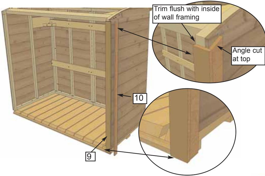
**16.** Close lid and mark the highest point **Front Corner Trims (9 & 9A)** 1/2" x 2 1/2" x 52" and **Front Side Corner Trim (10 & 10A)** with angle cut top 1/2" x 2 1/2" x 53" can be located without impeding the lid. Front trim should be positioned even with inside of wall framing. Attach each piece with **6 - 1 1/2" Finishing Nails (K)**.
