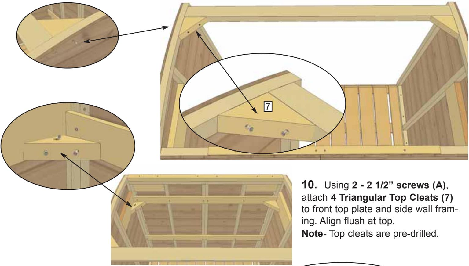
**10.** Using 2 - 2 1/2" screws (A), attach 4 **Triangular Top Cleats (7)** to front top plate and side wall framing. Align flush at top.
