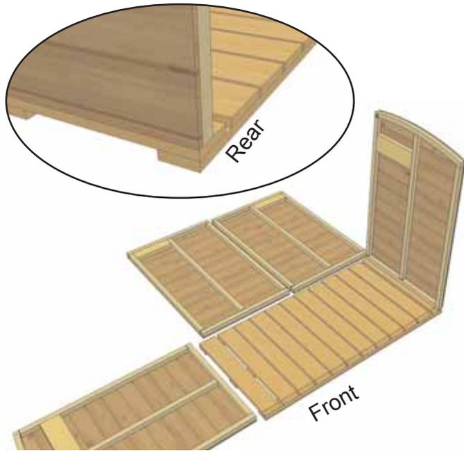
**3. Lift Side Wall (2)** up and orientate so wall framing is flush at rear with floor, wall siding is flush on side with floor. In the front, wall framing will overhang the floor as shown below.
