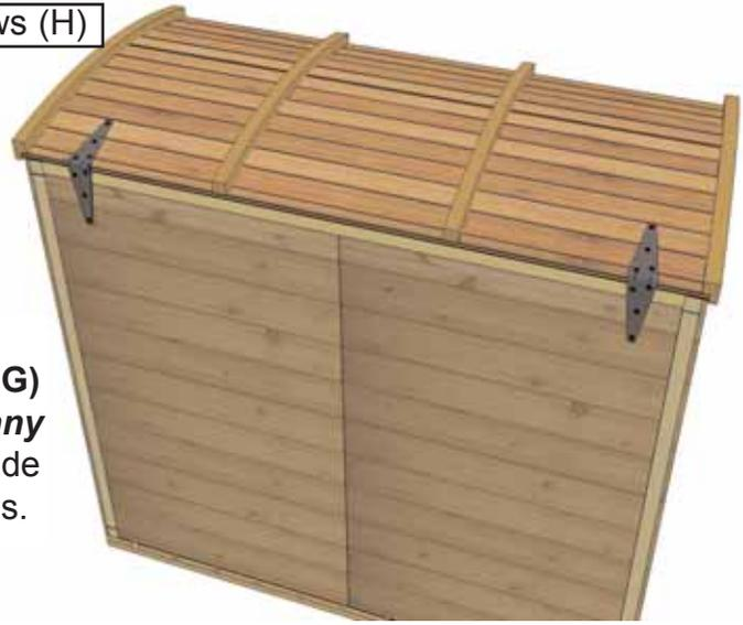
**13.** Complete Strap Hinge attachment using **1 - 1" Black Screw (F)** and **2 - 3/4" Black Screws (G)** on the lid side. *On the top wall side do not install any screws, leave the holes empty.* On the lower wall side install **2 - 2" Black Screws (H)**. Complete both sides.
