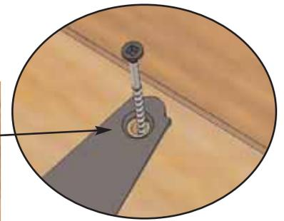
**12.** Locate both **Rear Black Strap Hinges (D)**. Orientate hinge as shown to right so pre-drilled hole in lid and top hinge hole align. Slide in a **2" Black Bolt with Washer and Nut (E)** through hinge hole and lid. From the inside, slide **Washer** on and tighten **Nut** snug with 3/8" socket or wrench. Complete both sides.
