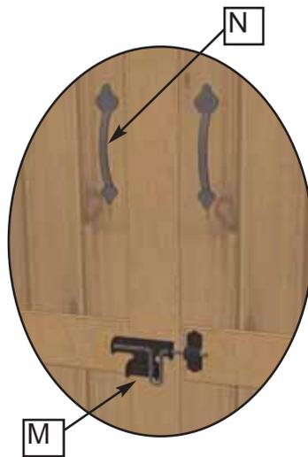
**23.** Position and attach **Black Barrel Bolt (M)** with **6 - 3/4" Black Screws (G)**. **Note** how female part of barrel bolt is positioned higher than male. Do a dry run first to position barrel bolt correctly. **Important** - Drill shallow pilot holes with 1/8" drill bit prior to securing with screws to prevent wood from splitting. Attach **2 Door Handles (N)** with **4 - 3/4" Black Screws (G)** per handle. Drill shallow pilot holes to prevent wood from splitting.
