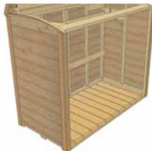
**18.** Center **Rear Trim (12)** 1/2" x 3 1/2" x 53" on rear wall seam and attach with **6 - 1 1/2" Finishing Nails (K)**. Align to same height and corner rear trims.
