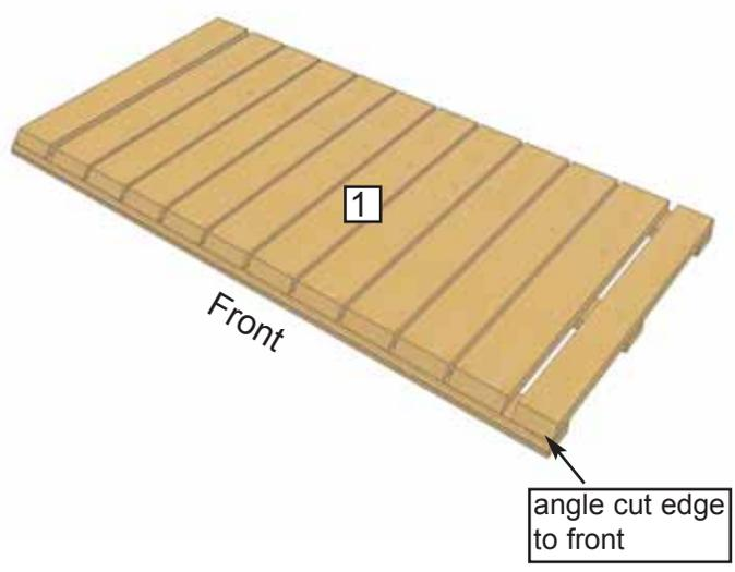
**1.** Locate **Floor (1)** and lay down on level foundation. Place floor with angle cut edge to the front. Level floor if required.
