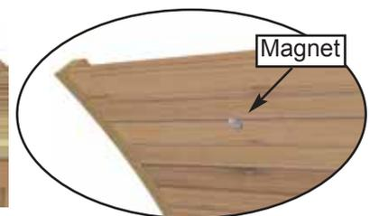
**26.** To complete, position and attach both **Lid Magnets (P)** to top of front top plate and to the underside of the lid. Start by attaching magnet bracket to inside edge of top plate with magnet screws. Close lid and mark location on the underside of the lid. Try using duct tape (sticky side up) on bracket magnet to help with alignment. Attach to lid with magnet screws.
