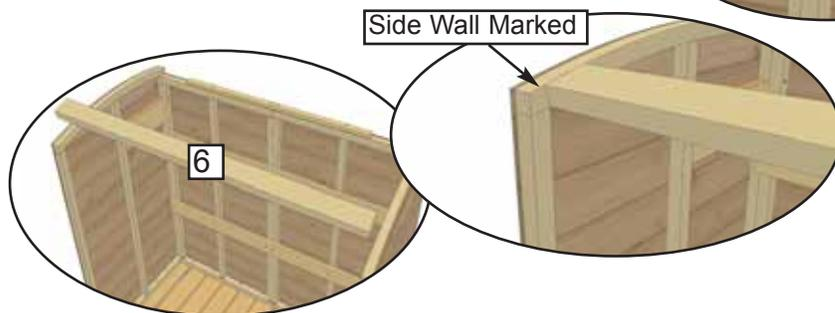
**9. Place Front Top Plate (6)** between side walls at top front. Side walls will be marked for plate alignment on the inside framing. With you helpers holding one end, secure opposite end with **2 - 3" screws (C)**. Side walls are pre-drilled. Complete both ends.
