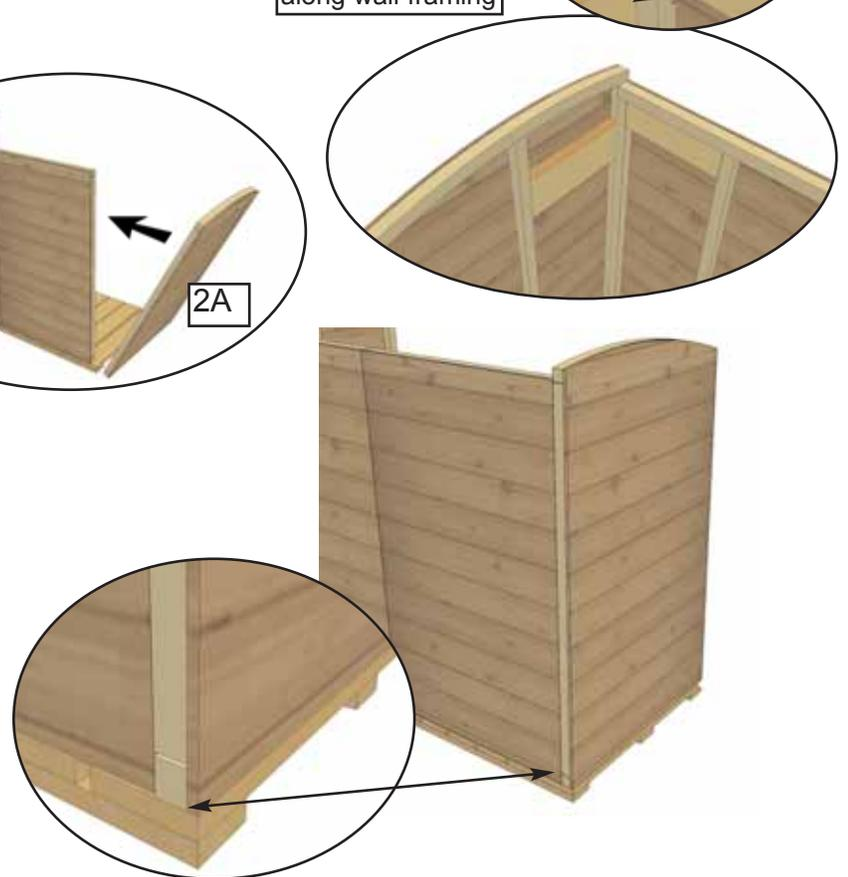
**7.** Check for wall/floor alignment (wall siding flush with outside of floor on sides and rear). When satisfied, secure wall framing to floor with **4 - 2 1/2" screws (A)** per wall panel.
