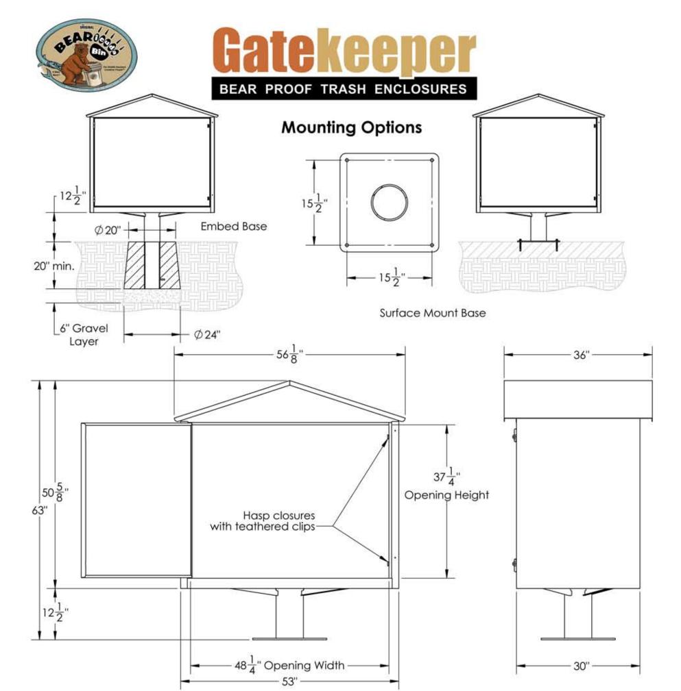
The Gatekeeper Enclosure is designed to enclose three 30 gallon rectangular trash cans. The access door is equipped with two hasps, upper and lower. Clips, teathered by cables, are used to secure the hasps and thwart entry by woodland creatures and neighborhood pets. Solid 14 gauge steel construction coupled with an extra durable powder coating shell ensure long lasting utility and beauty. These rugged enclosures are also available in either a surface mount or embedded configuration.
