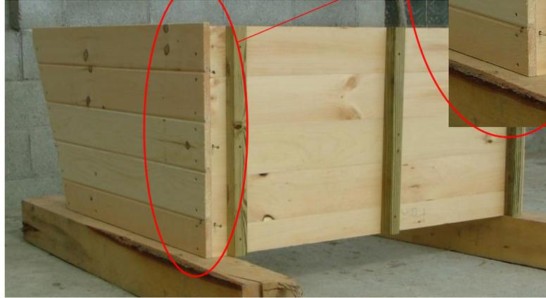
Rear attached in two pieces. Each piece is attached to the two ends and the floor using three 1-5/8" screws on the bottom and seven to eight running up the sides.
